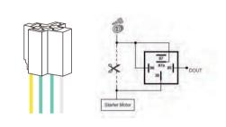
12V relay is standard. The device is suitable for vehicles with 12V supply. If the vehicle power supply is 24V, use 24V relay.
