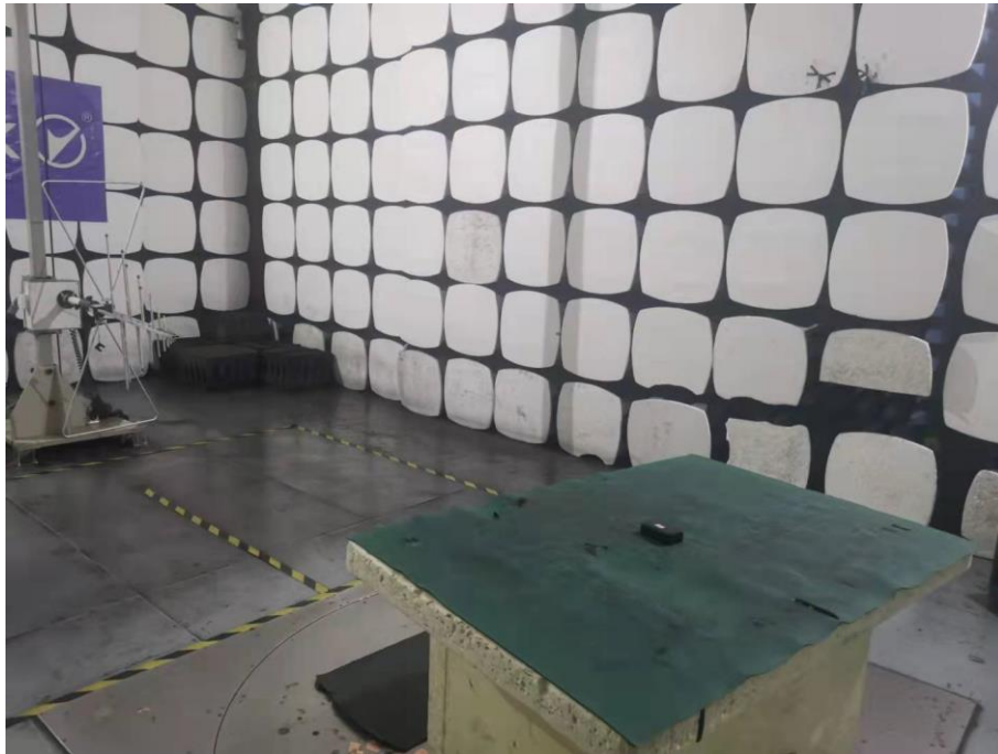
Spurious Emission Test Setup (Below 1GHz)
