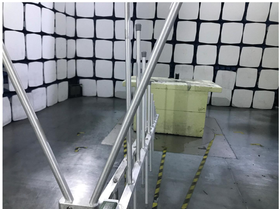
Radiation Emission Test Setup (30MHz to 1GHz)
