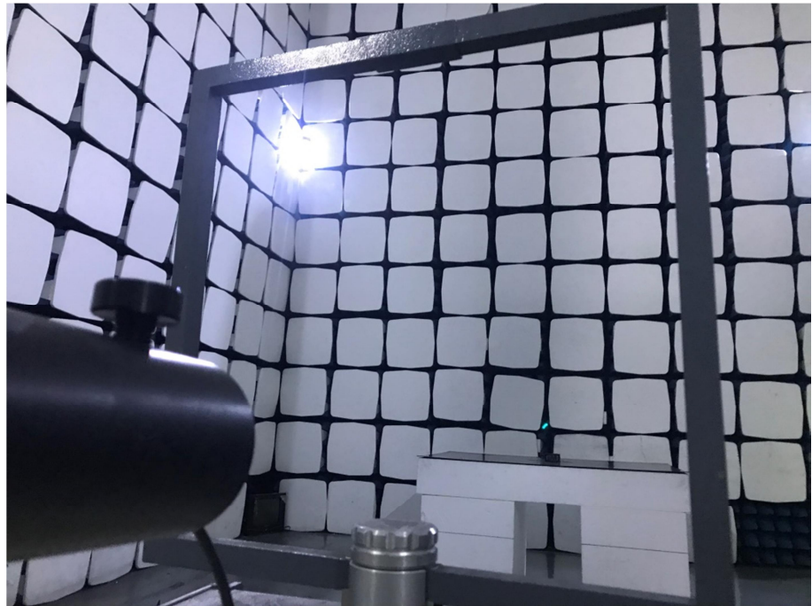
Radiation Emission Test Setup (Below 30MHz)
