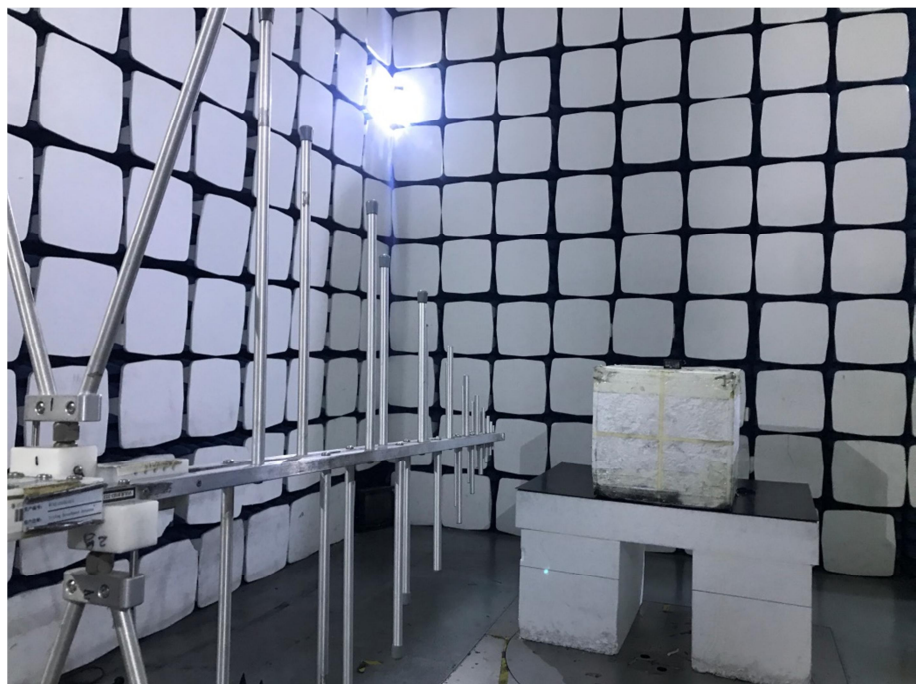
Radiation Emission Test Setup (30MHz to 1GHz)
