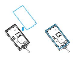
5. Press the upper case down and make sure all 5 clips are completely in place.
