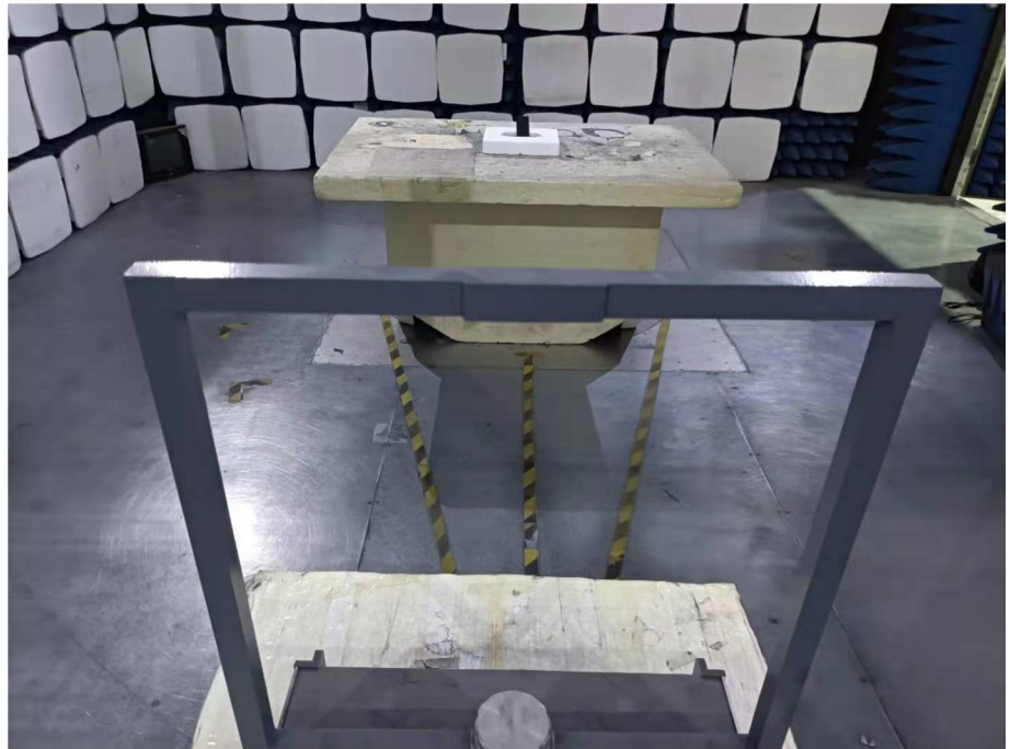
Radiation Emission Test Setup (Below 30MHz)
