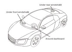
1) The device should face up to the sky. 2) Metal thermal barrier or heating layer of the windshield affects the signal.
