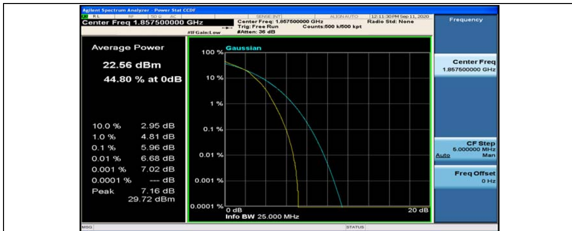
(Channel Bandwidth:15 MHz)_LCH_16QAM_37RB#18
