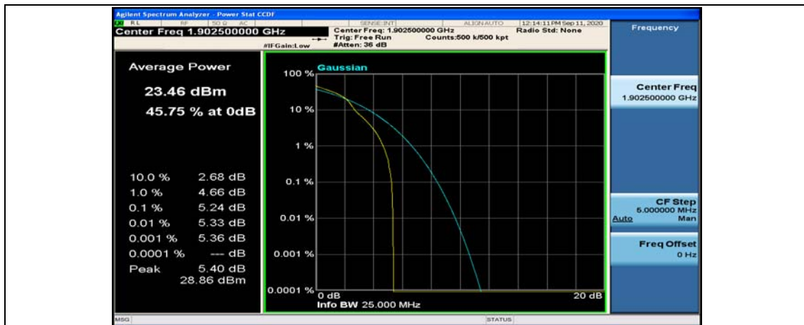
(Channel Bandwidth:15 MHz)_HCH_16QAM_1RB#74
