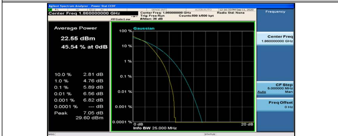
(Channel Bandwidth:20 MHz)_LCH_16QAM_100RB#0
