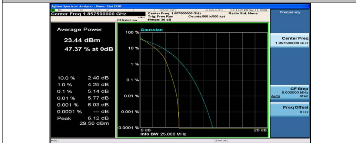
(Channel Bandwidth:15 MHz)_LCH_QPSK_75RB#0
