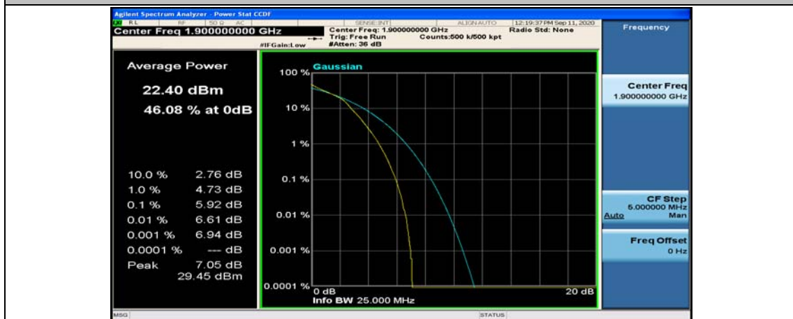
(Channel Bandwidth:20 MHz)_HCH_16QAM_50RB#25
