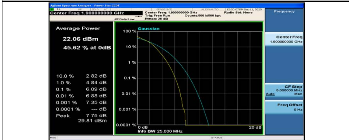
(Channel Bandwidth:20 MHz)_HCH_16QAM_100RB#0
