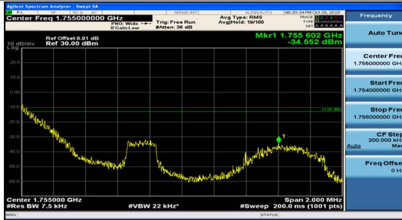
(Channel Bandwidth: 1.4 MHz)_HCH_16QAM_1RB#3
