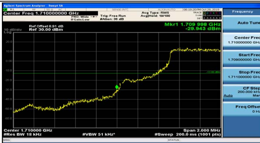
(Channel Bandwidth: 1.4 MHz)_LCH_QPSK_3RB#3
