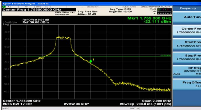
(Channel Bandwidth: 5 MHz)_HCH_QPSK_12RB#0
