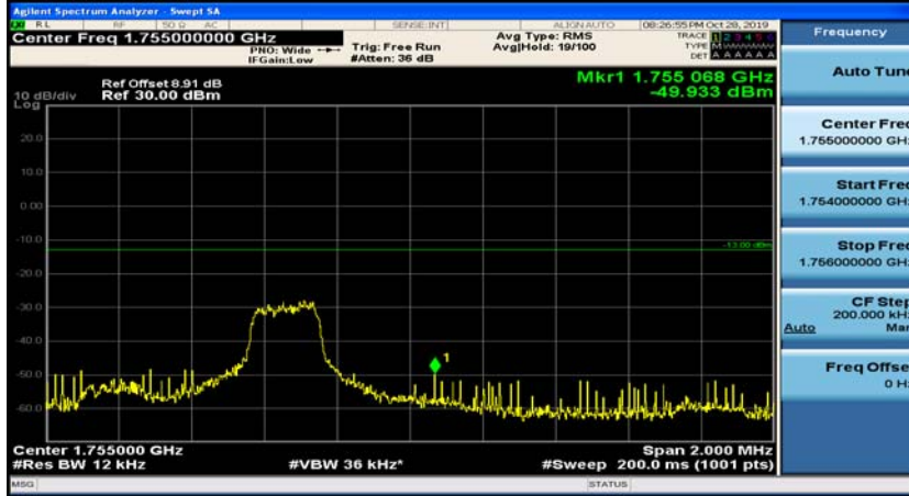
(Channel Bandwidth: 5 MHz)_HCH_QPSK_1RB#12
