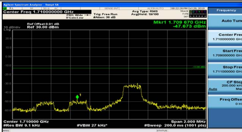
(Channel Bandwidth: 3 MHz)_LCH_16QAM_8RB#0
