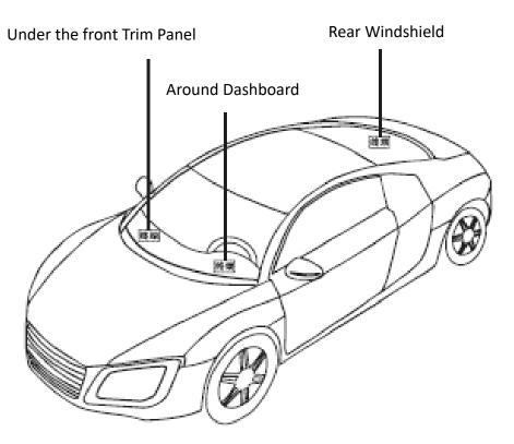
**Note:** The device should be installed face up to the sky. If the windshield is pasted with a metal thermal insulation layer or a heating layer, it will reduce the signal strength of the satellite, which may make it difficult to locate the satellite. Please change the installation location.
