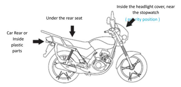
Note: the satellites signal will greatly degrade if be installed under the driver
