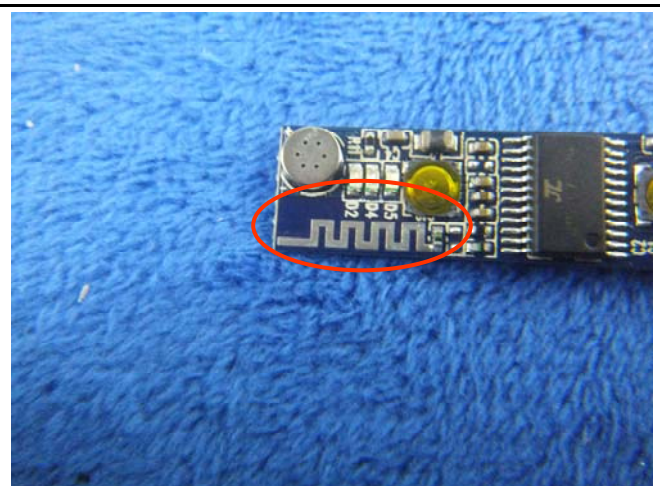
BT - Antenna View
