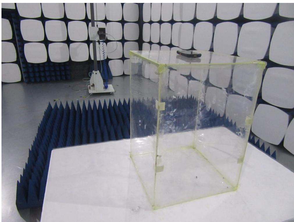
**Radiated Spurious Emission Test Setup FOR (PCE )**
