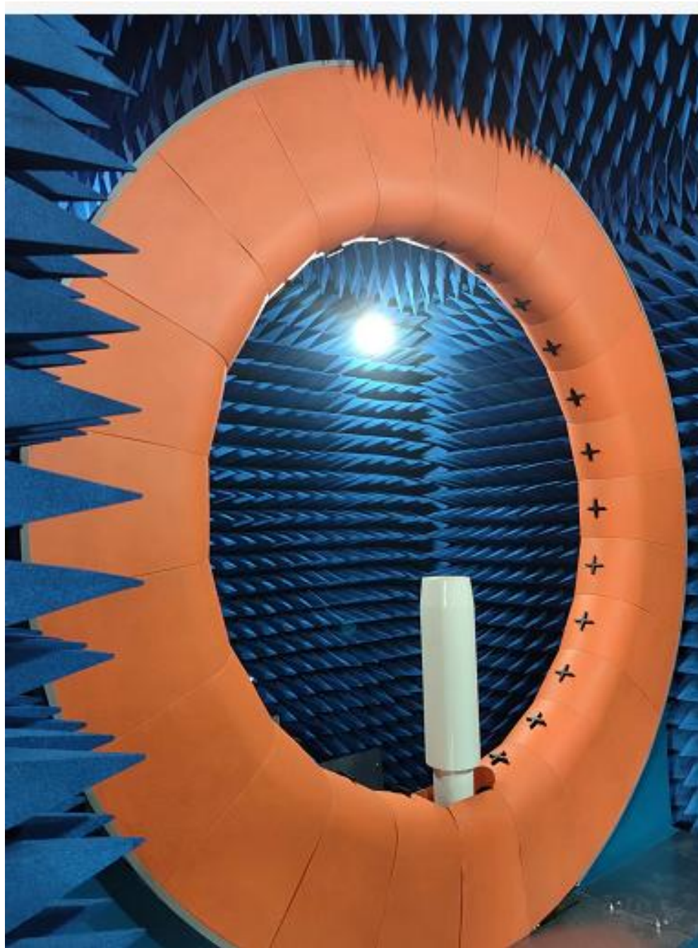
24 probe microwave anechoic chamber test equipment
