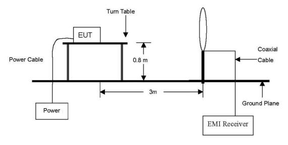
The diagram below shows the test setup that is utilized to make the measurements for emission from 30 Number 12 Numb to 1 GHz.
