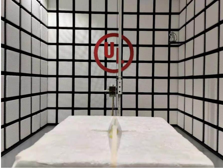
RADIATED RF MEASUREMENT SETUP (30MHz~1GHz)
