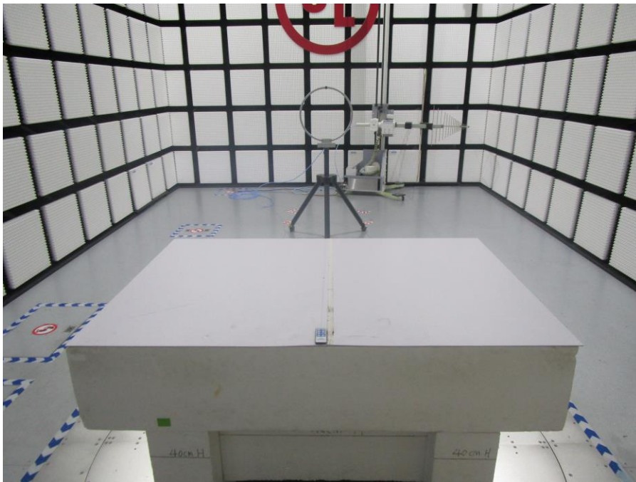
RADIATED RF MEASUREMENT SETUP (30MHz~1GHz)
