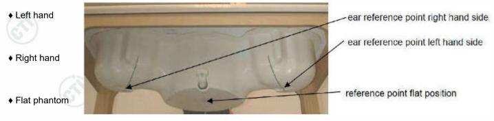
The phantom table for the DASY systems have the size of  $100 \times 50 \times 85$  cm (L xWx H). these tables are reinforced for mounting of the robot onto the table. For easy dislocation these tables have fork lift cut outs at the bottom.
