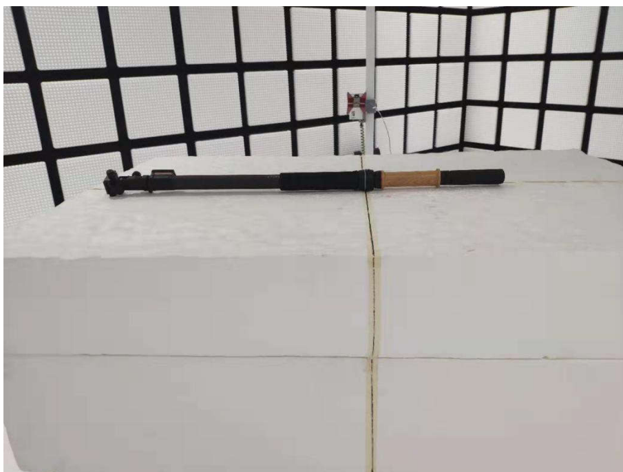
Radiated spurious emission Test Setup-3(Above 1GHz)
