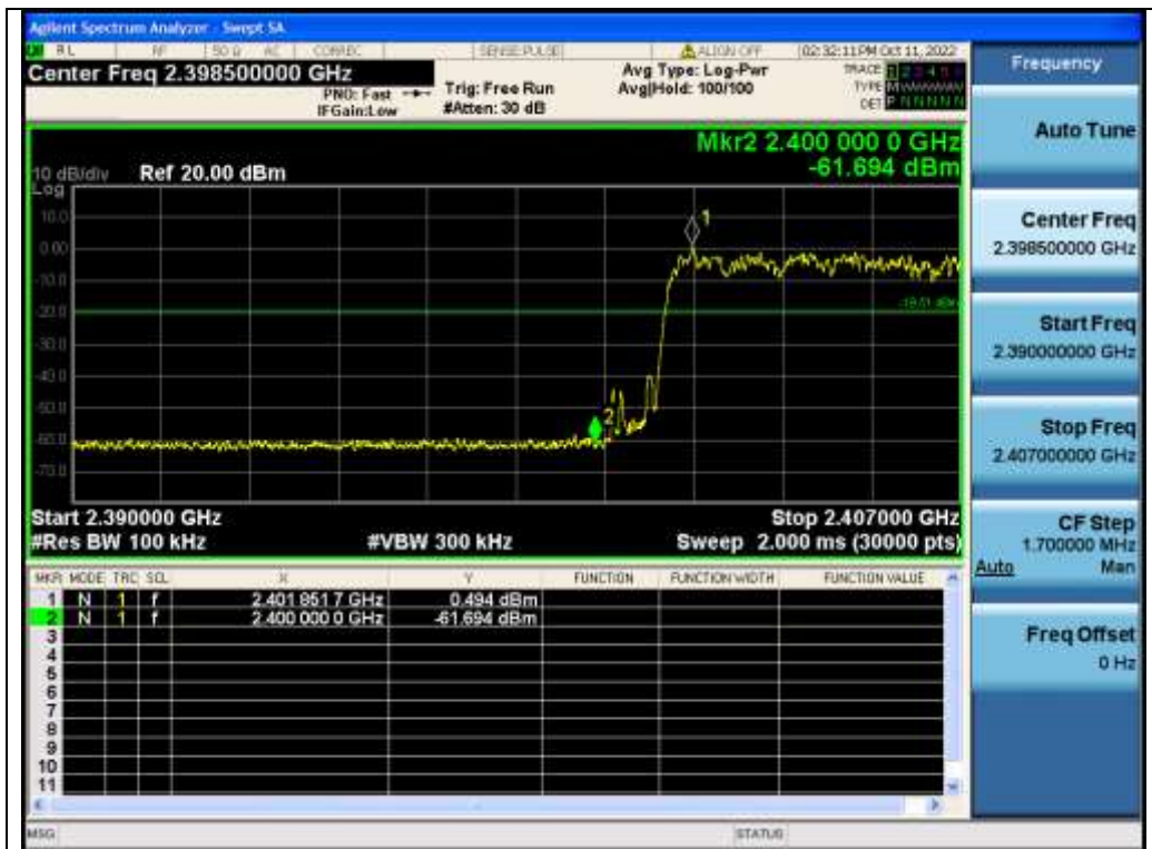
Test_Graph_EDR_HOP_ANT1_NA_3Mbps_Lower Band Edge Emissions
