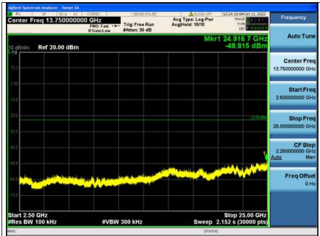
Test_Graph_BR_ANT1_2480_1Mbps_Higher Band Emissions
