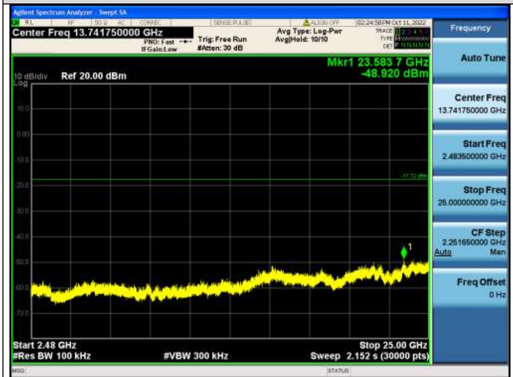
Test_Graph_EDR_ANT1_2441_3Mbps_Higher Band Emissions
