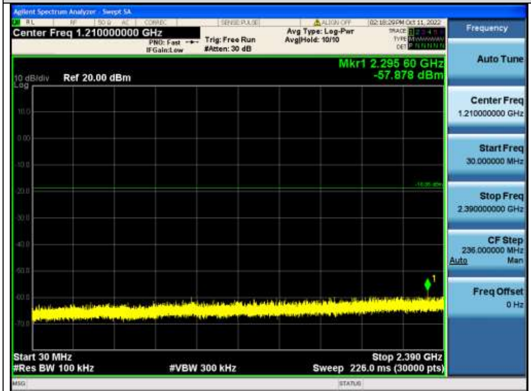
Test_Graph_EDR_ANT1_2402_3Mbps_Lower Band Emissions
