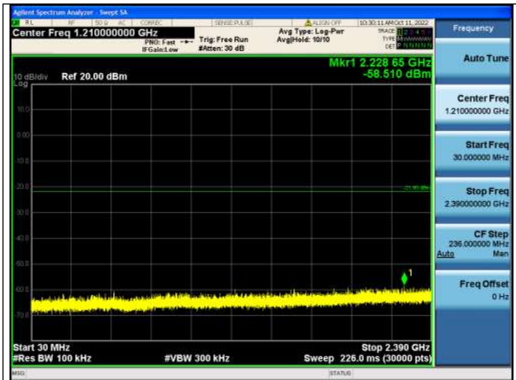
Test_Graph_EDR_ANT1_2402_2Mbps_Lower Band Emissions
