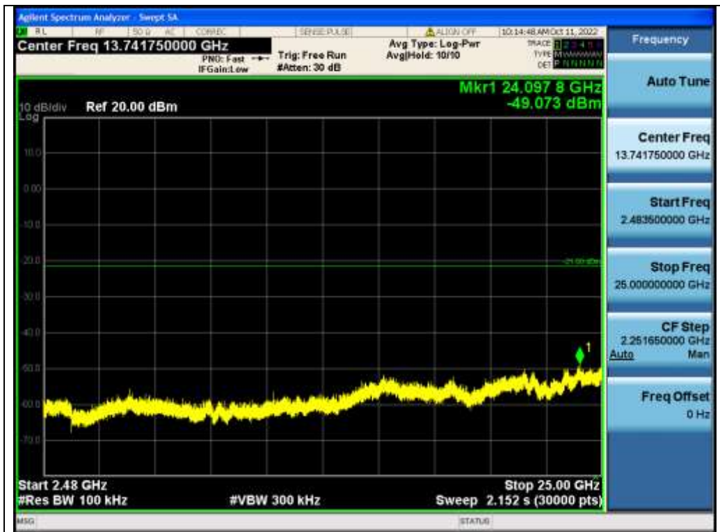
Test_Graph_BR_ANT1_2402_1Mbps_Higher Band Emissions
