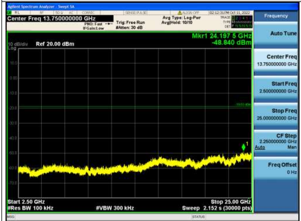
Test_Graph_EDR_ANT1_2480_2Mbps_Higher Band Emissions
