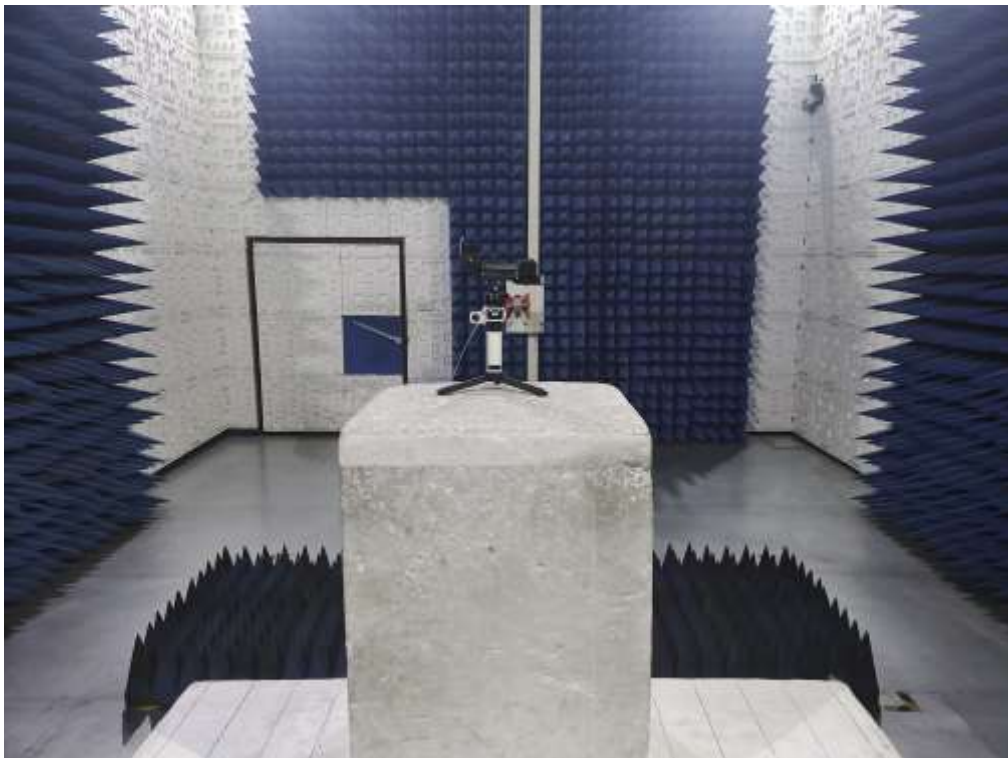
RADIATED EMISSION TEST SETUP ABOVE 1GHz
