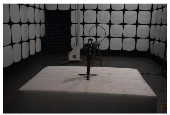
3. Radiated emission (9KHz-30MHz)
