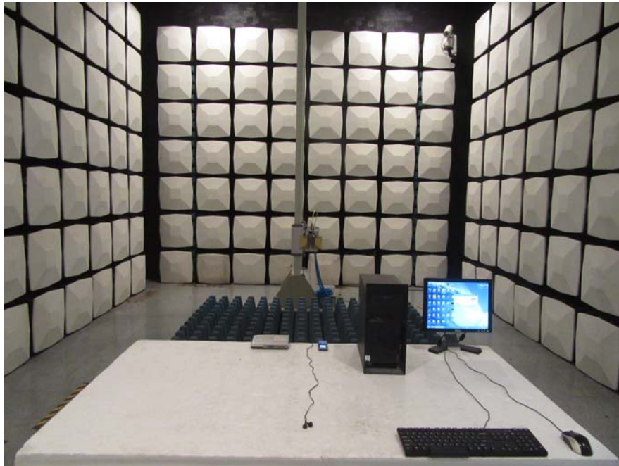
Radiated Emission - Front View (Above 1 GHz)
