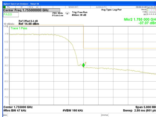
A8 FIELD STRENGTH OF SPURIOUS RADIATION MEASUREMENT
