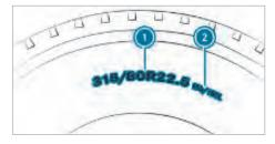
Example: tyre size and load-bearing index
