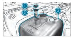
Hydraulic fluid reservoir (3) is either a single tank on the right-hand side of the vehicle or combined with the fuel tank on the left-hand side of the vehicle as a combination tank.
