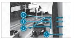
The overtaking assistant is an extended display of the distance lines. The function is intended to support the driver in overtaking on roads with several lanes in the direction of travel.
