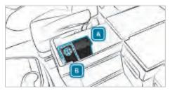
Use the waste receptacle only in position A or B. Otherwise, the waste receptacle will not be secured and may tip over during a journey.
