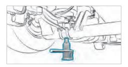
Position the jack under the axle tube, between the mounting brackets.
