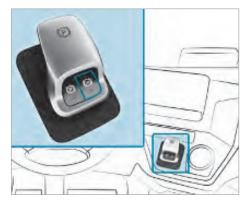
TSA button on the electric parking brake lever (example)
