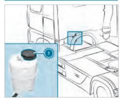
Before commencing your journey, the oil level should be checked with the hydraulic system cold, at an oil temperature of about 20 °C.
