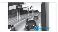
After switching on the ignition or after changing the semitrailer/trailer, adjustable distance line shown in the display can be moved to the back edge of the trailer/semitrailer.
