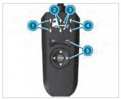
Example: control panel for fully air-sprung vehicles
