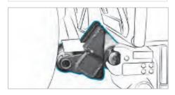
Tipper with air suspension in road paver mode (overrun mode)
