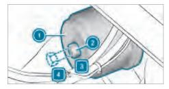
Spring-loaded brake cylinder with release screw
