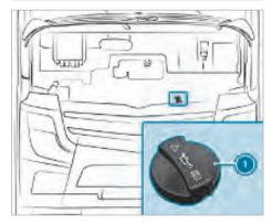
Only top up the oil filling capacity displayed on the on-board computer when the <u>symbol</u> appears in the menu window.
