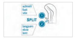
The splitter box allows you to select a slow or fast ratio of the selected gear without changing the gear itself.
