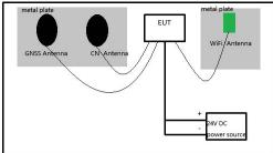
3. The EUT shall be replaced by a substitution antenna. The test setup refers to figure below.
