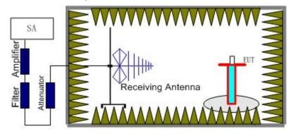
2. The EUT is then put into continuously transmitting mode at its maximum power level during the test. And the maximum value of the receiver should be recorded as (Pr). The placement of EUT is shown in the figure below:
