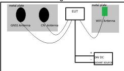
3. The EUT was tested in two states, horizontal and vertical.as show in the attachment. Additionally, during the testing, the WLAN which worked on 802.11b channel 6 (Power level is
