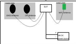
3. The EUT was tested in two states, horizontal and vertical.as show in the attachment.
