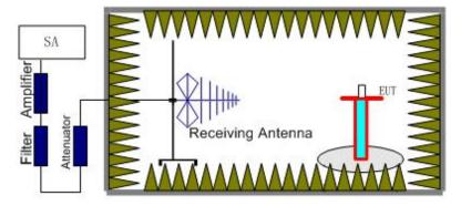
2. The EUT is then put into continuously transmitting mode at its maximum power level during the test. And the maximum value of the receiver should be recorded as (Pr). The placement of EUT and AE is shown in the figure below:
