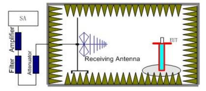
2. The EUT is then put into continuously transmitting mode at its maximum power level during the test. And the maximum value of the receiver should be recorded as (Pr). The placement of
