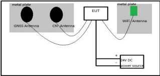
3. The EUT was tested in two states, horizontal and vertical.as show in the attachment.
