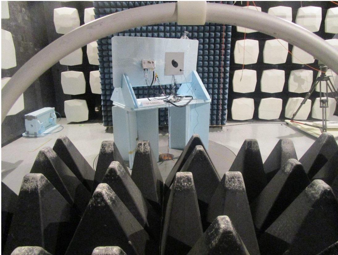
H-field measurement in Semi anechoic room
