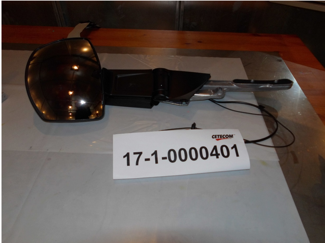
Photograph 7: external GPS antenna
