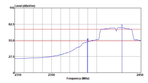
Mode:a; Polarization:Horizontal; Modulation:n; bandwidth:40MHz; Channel:Low
