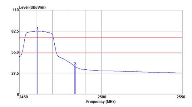
Mode:a; Polarization:Vertical; Modulation:g; bandwidth:20MHz; Channel:High
