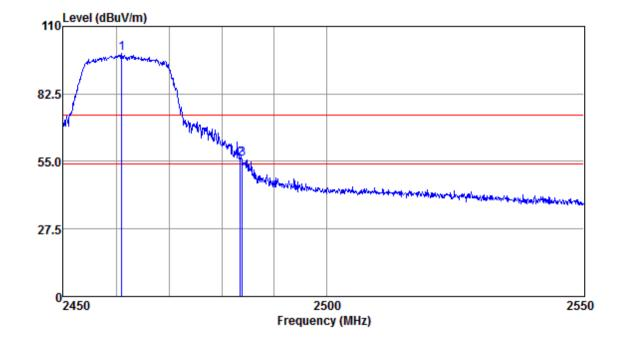
Mode:a; Polarization:Vertical; Modulation:g; bandwidth:20MHz; Channel:High
