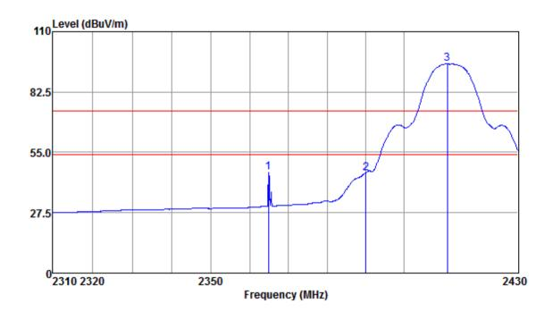
Mode:a; Polarization:Horizontal; Modulation:b; bandwidth:20MHz; Channel:Low
