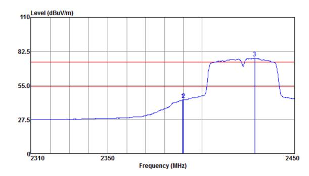
Mode:a; Polarization:Vertical; Modulation:n; bandwidth:40MHz; Channel:Low
