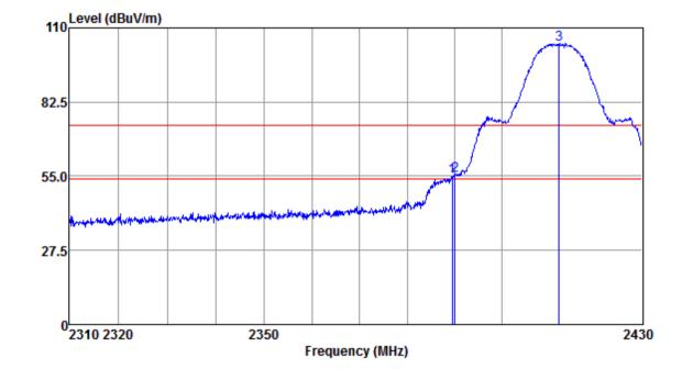
Mode:a; Polarization:Horizontal; Modulation:b; bandwidth:20MHz; Channel:Low
