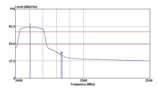
Mode:a; Polarization:Vertical; Modulation:n; bandwidth:20MHz; Channel:High
