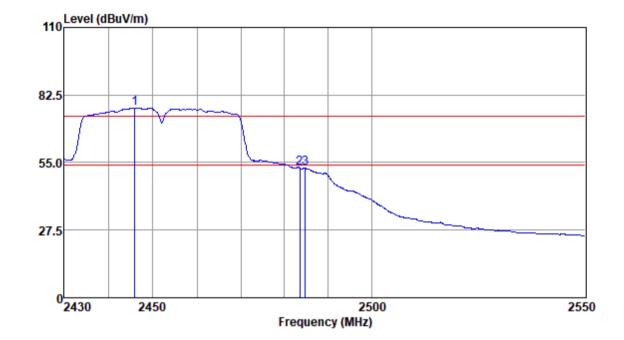
Mode:a; Polarization:Horizontal; Modulation:n; bandwidth:40MHz; Channel:High
