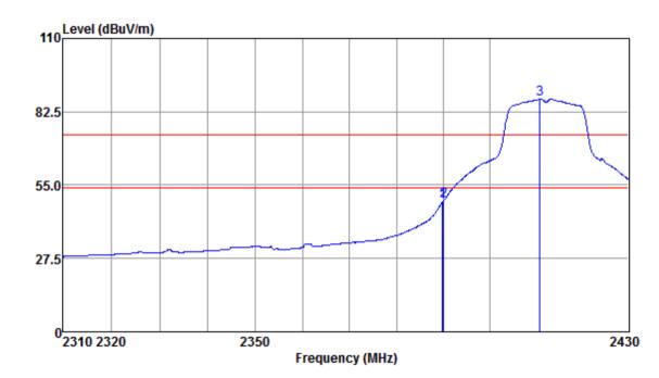
Mode:a; Polarization:Horizontal; Modulation:g; bandwidth:20MHz; Channel:Low
