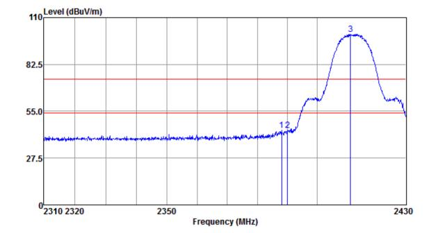
Mode:a; Polarization:Vertical; Modulation:b; bandwidth:20MHz; Channel:Low
