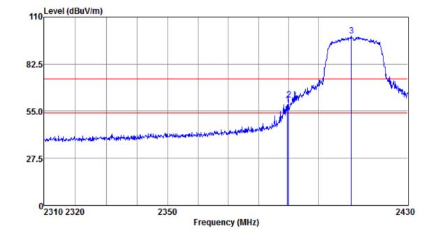
Mode:a; Polarization:Vertical; Modulation:n; bandwidth:20MHz; Channel:Low
