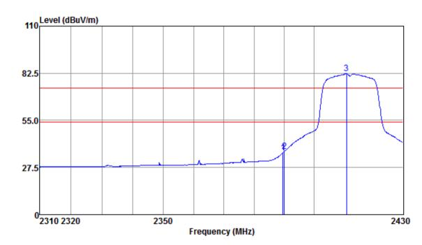
Mode:a; Polarization:Vertical; Modulation:n; bandwidth:20MHz; Channel:Low
