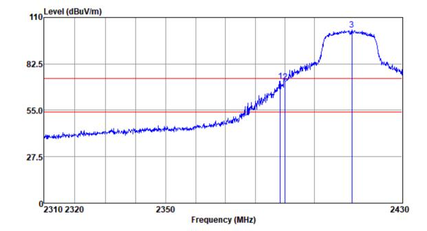
Mode:a; Polarization:Horizontal; Modulation:n; bandwidth:20MHz; Channel:Low
