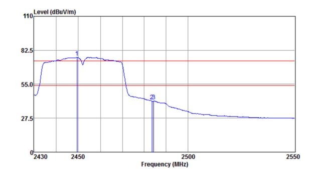
Mode:a; Polarization:Vertical; Modulation:n; bandwidth:40MHz; Channel:High
