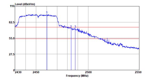
Mode:a; Polarization:Horizontal; Modulation:n; bandwidth:40MHz; Channel:High
