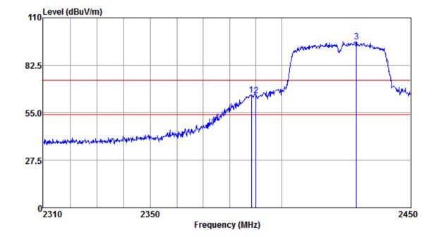
Mode:a; Polarization:Vertical; Modulation:n; bandwidth:40MHz; Channel:Low
