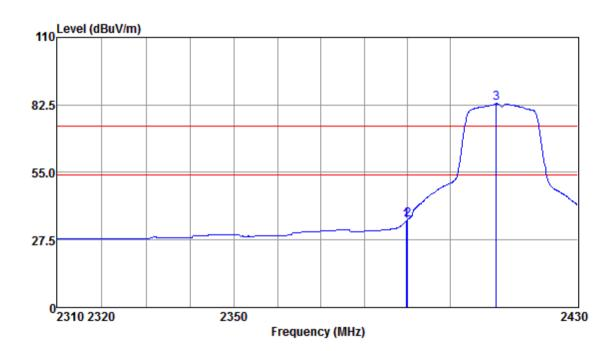
Mode:a; Polarization:Vertical; Modulation:g; bandwidth:20MHz; Channel:Low
