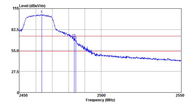
Mode:a; Polarization:Horizontal; Modulation:g; bandwidth:20MHz; Channel:High
