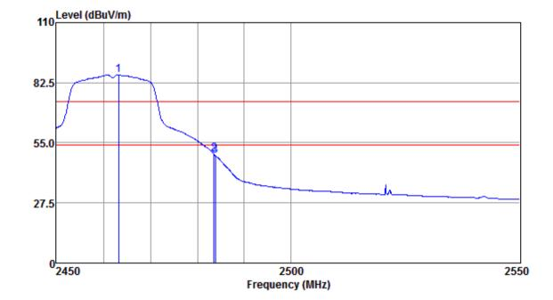
Mode:a; Polarization:Horizontal; Modulation:n; bandwidth:20MHz; Channel:High
