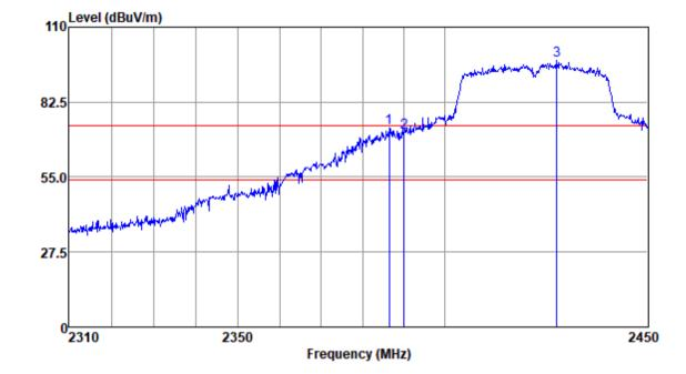
Mode:a; Polarization:Horizontal; Modulation:n; bandwidth:40MHz; Channel:Low
