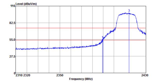
Mode:a; Polarization:Vertical; Modulation:g; bandwidth:20MHz; Channel:Low
