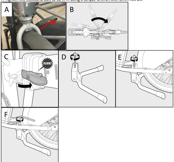
△ Warning: Failure to not secure the kickstand properly could cause it to fall off during riding.
