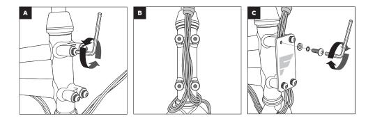
Note: Following installation of the front logo plate, check that the cables and wires can move freely by turning the handlebars fully to either side. If any resistance occurs, the wires and cables should be repositioned by sliding them up or down along the headtube.
