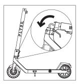
**Step 1**Rotate the tube to the vertical position.
