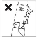
$\triangle$  WARNING: Failure to follow unfolding instructions could result in unintentional folding. Ensure that the lever is upright and the sleeve is locked in place.
