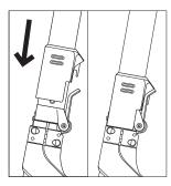
**Step 3**Slide the locking sleeve down until it is fully seated.
