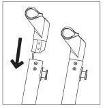
**Step 5**Slide the handlebar assembly into the tube. Push the handle bar assembly down until it is fully seated.
