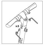
**Step 6**Install four screws to the top of the tube using the provided Hex wrench. Tighten the screws until they are snug.
