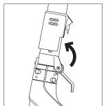
**Step 2**Rotate the lever up while holding the tube in place.
