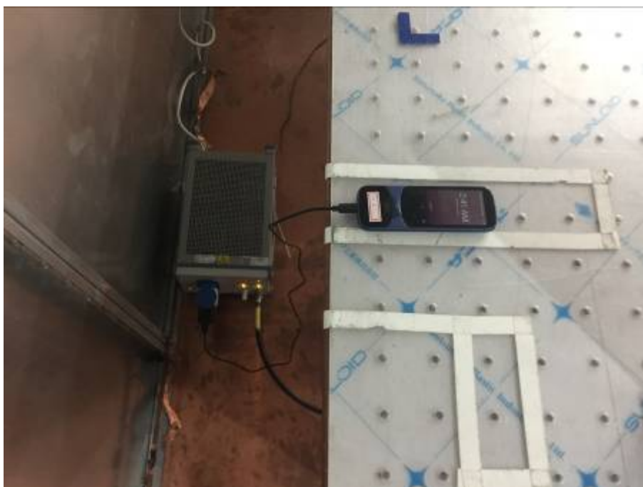
Conducted Emissions Test Setup (with charger)
