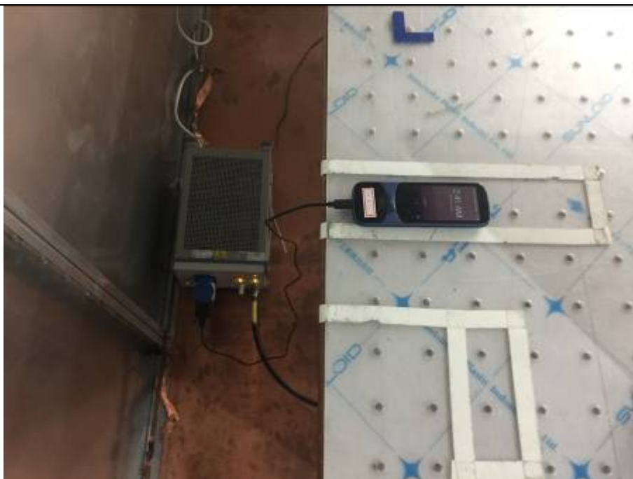
Conducted Emissions Test Setup (with charger)
