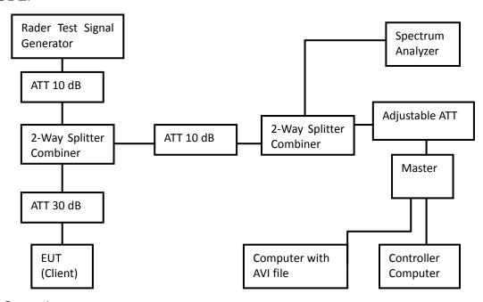
**Test Setup Operation**
