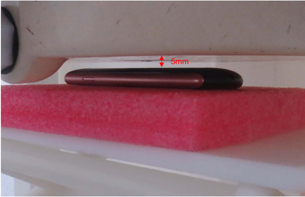
Back Side, the distance from handset to the bottom of the Phantom is 5mm
