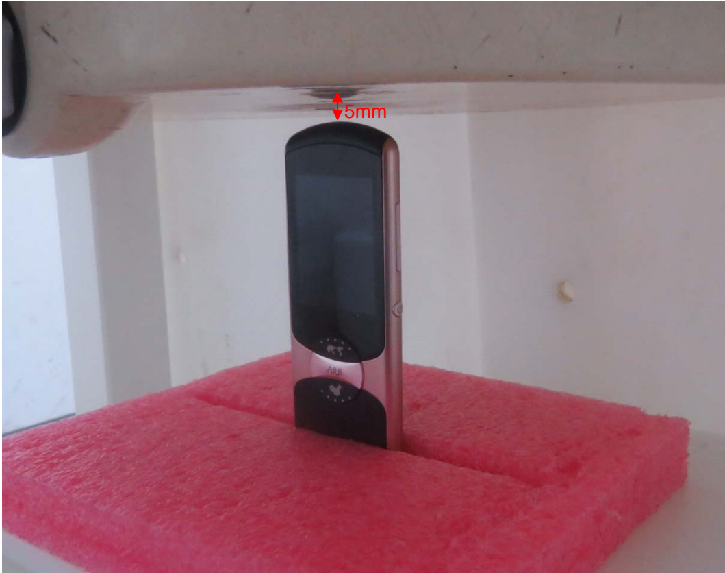
Top Edge, the distance from handset to the bottom of the Phantom is 5mm
