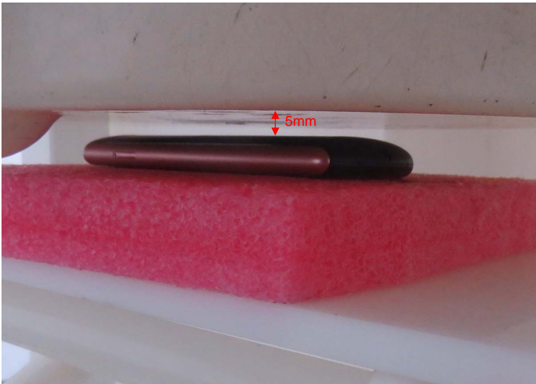
Front Side, the distance from handset to the bottom of the Phantom is 5mm
