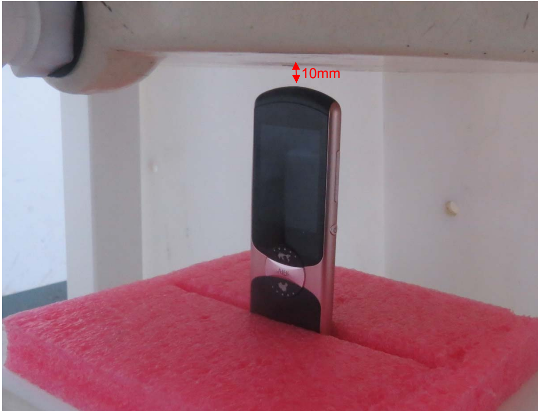
Picture 10: Top Side, the distance from handset to the bottom of the Phantom is 10mm
