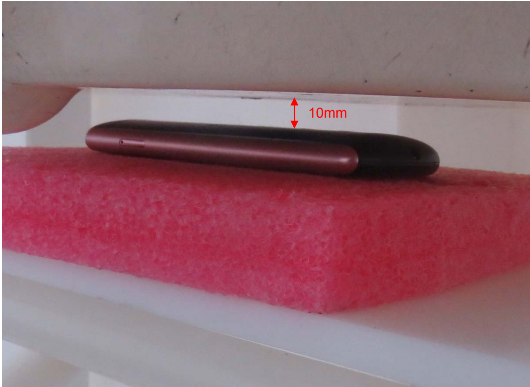
Picture 6: Back Side, the distance from handset to the bottom of the Phantom is 10mm
