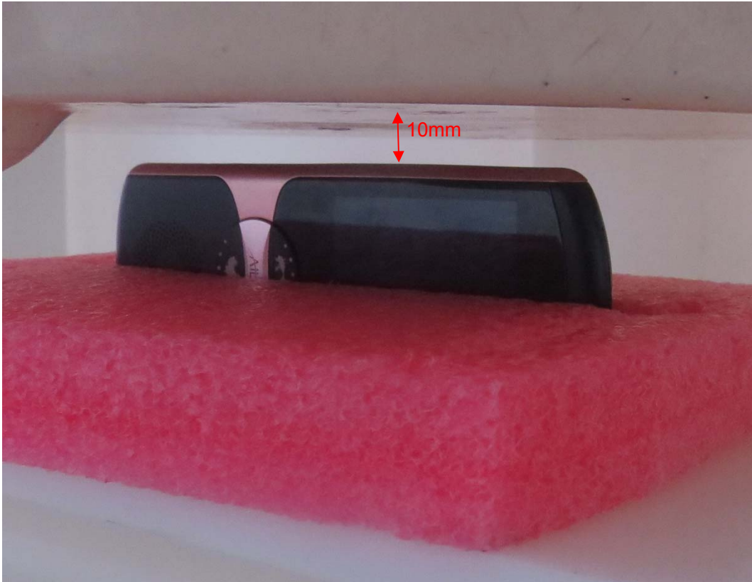
Picture 8: Left Side, the distance from handset to the bottom of the Phantom is 10mm
