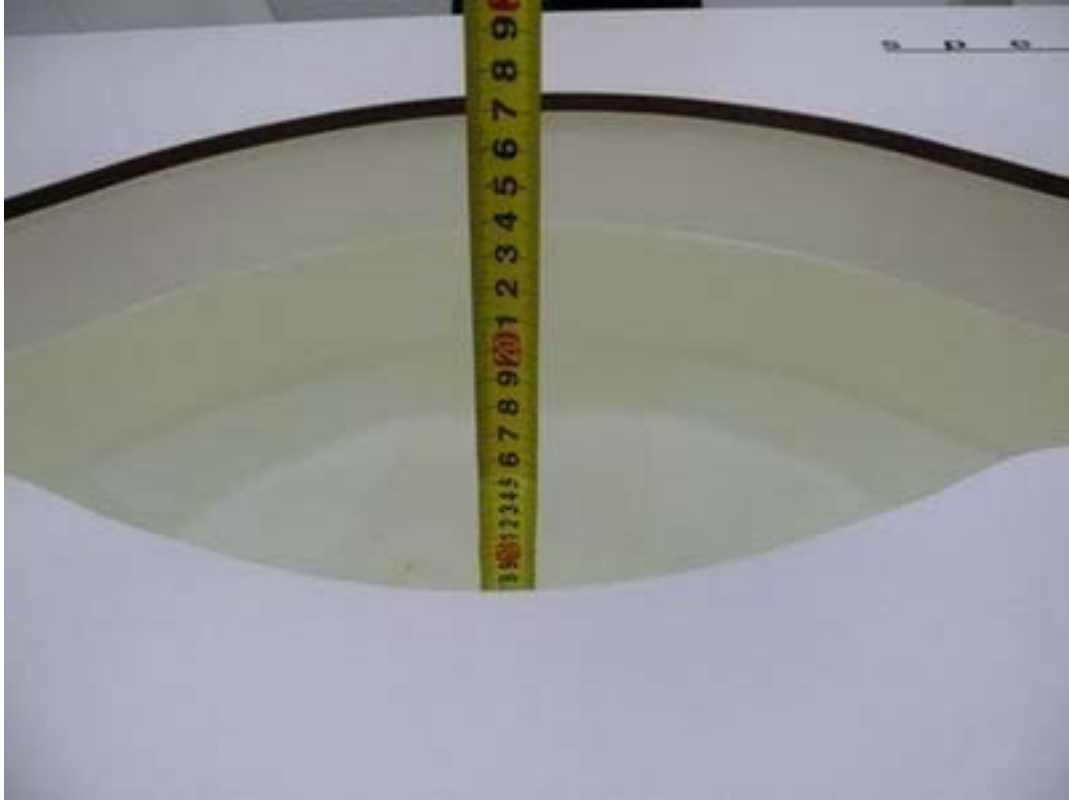
Picture 3: Liquid depth in the flat Phantom (5250 MHz, 15.3cm depth)
