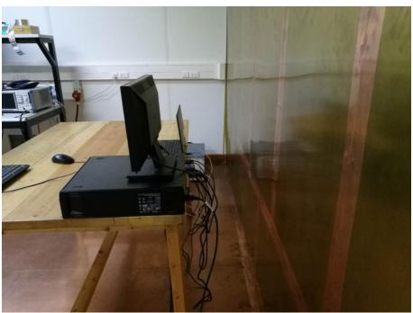
Test Mode: Mode 2 Description: Radiated Emission Test Setup
