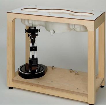
The ELI4 Phantom also is a fiberglass shell phantom with 2mm shell thickness. It has 30 liters filling volume, and with a dimension of 600mm for major ellipse axis, 400mm for minor axis. It is intended for compliance testing of handheld and body-mounted wireless devices in frequency range of 30 MHz to 6GHz. ELI4 is fully compatible with standard and all known tissue simulating liquids.
