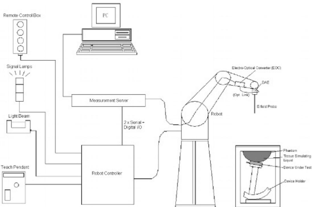
**Figure 2.1 SPEAG DASY5 System Configurations**
