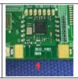
The antenna is PCB antenna. The best case gain of the antenna is 0.3dBi.
