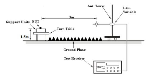
The radiated emission tests were performed in the 3 meters test site, using the setup accordance with the ANSI C63.10 - 2013. The specification used was the FCC 15 § 15.209, 15.205 and 15.231.
