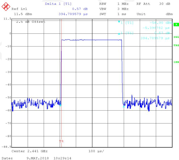
**BDR (GFSK): Pulse time, High Channel, DH1**
