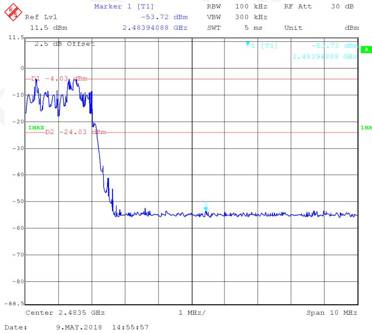
**EDR (8DPSK): Left Side - Hopping**
