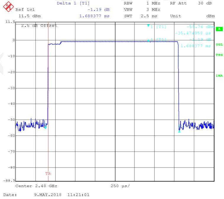
**EDR (8DPSK): Pulse time, Low Channel, 3DH5**
