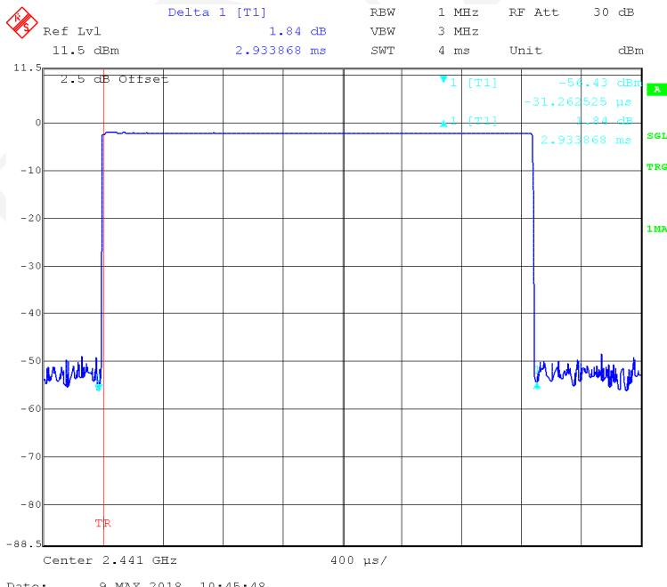
**BDR (GFSK): Pulse time, High Channel, DH5**
