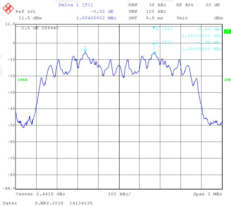
**EDR ( $\pi/4$ -DQPSK): High Channel**
