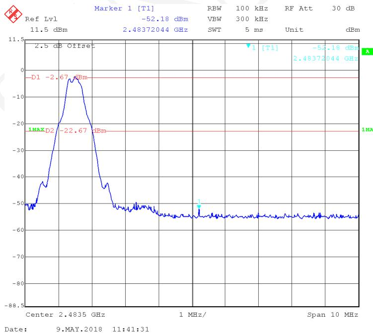
**EDR ( $\pi/4$ -DQPSK): Left Side**
