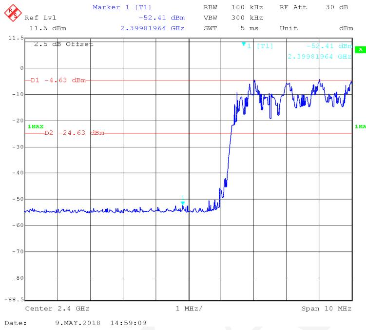
**EDR ( $\pi/4$ -DQPSK): Right Side - Hopping**
