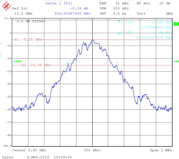
**EDR ( $\pi/4$ -DQPSK): Low Channel**
