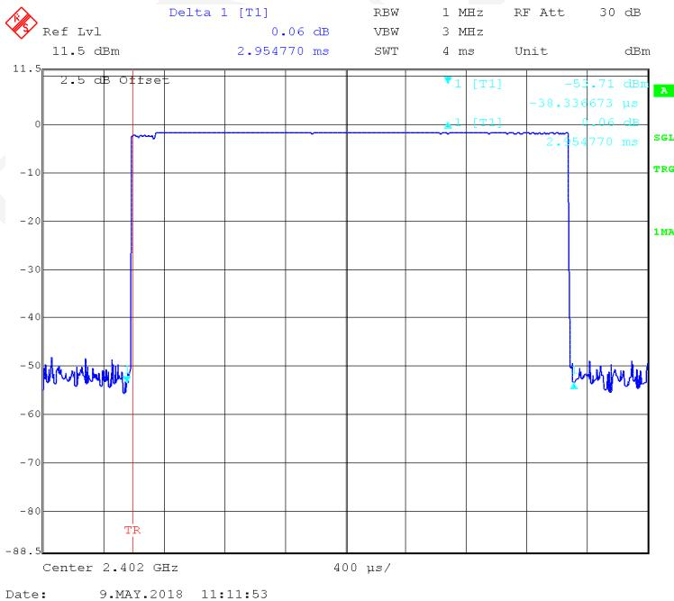
**EDR ( $\pi/4$ -DQPSK):Pulse time, Middle Channel, 2DH5**
