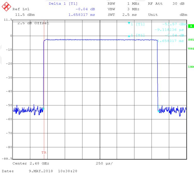
**BDR (GFSK): Pulse time, Low Channel, DH5**
