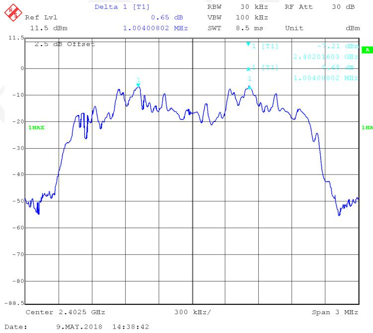
**EDR (8DPSK): Middle Channel**
