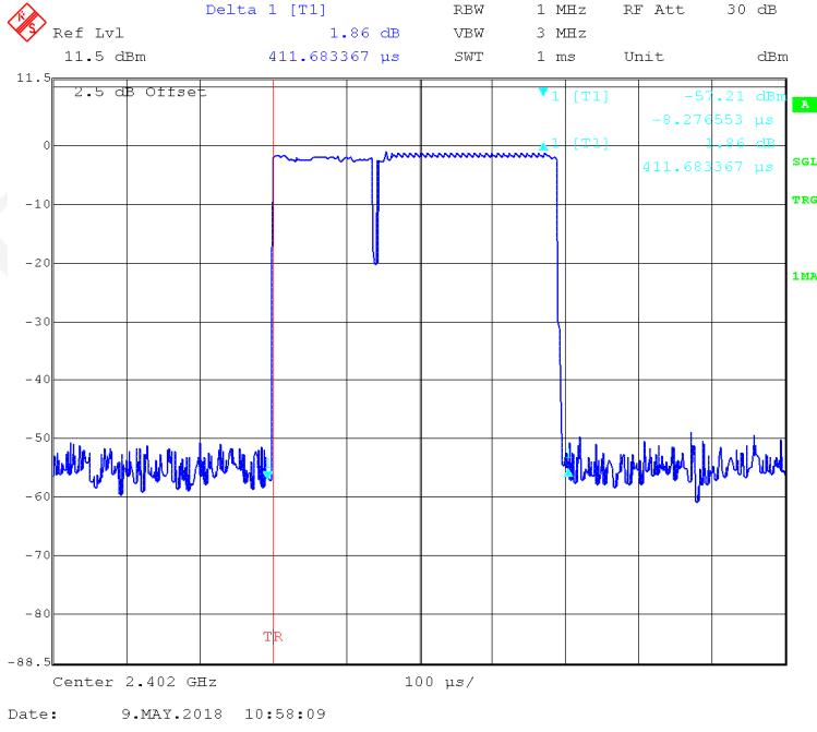
**EDR ( $\pi/4$ -DQPSK):Pulse time, Middle Channel, 2DH1**
