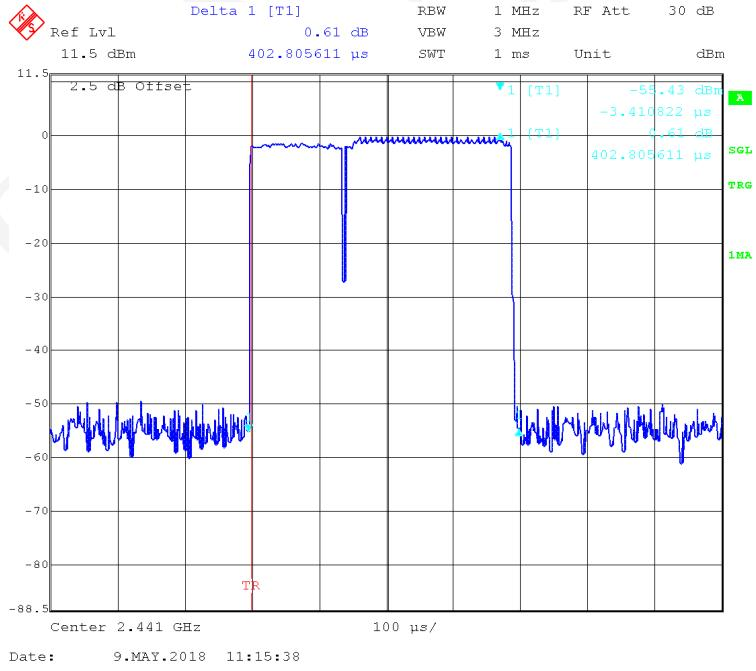
**EDR (8DPSK): Pulse time, High Channel, 3DH1**
