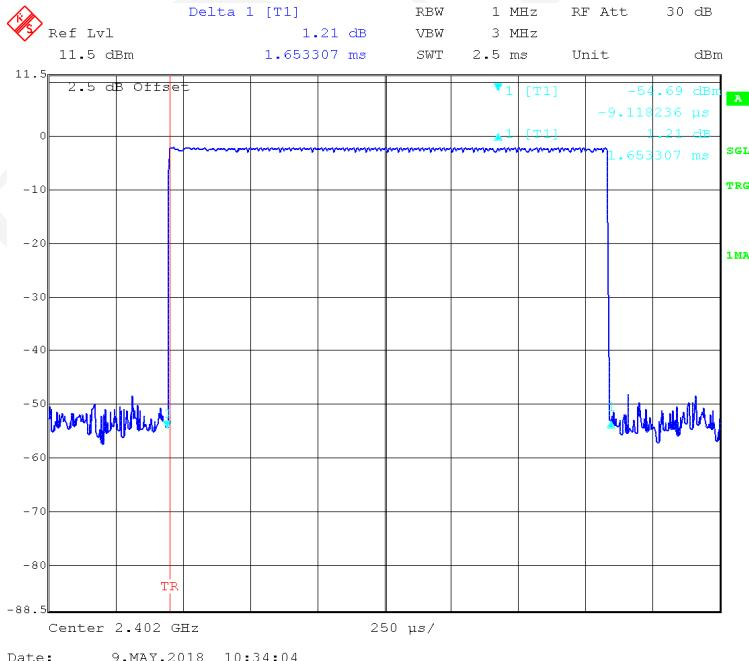
**BDR (GFSK): Pulse time, Middle Channel, DH3**
