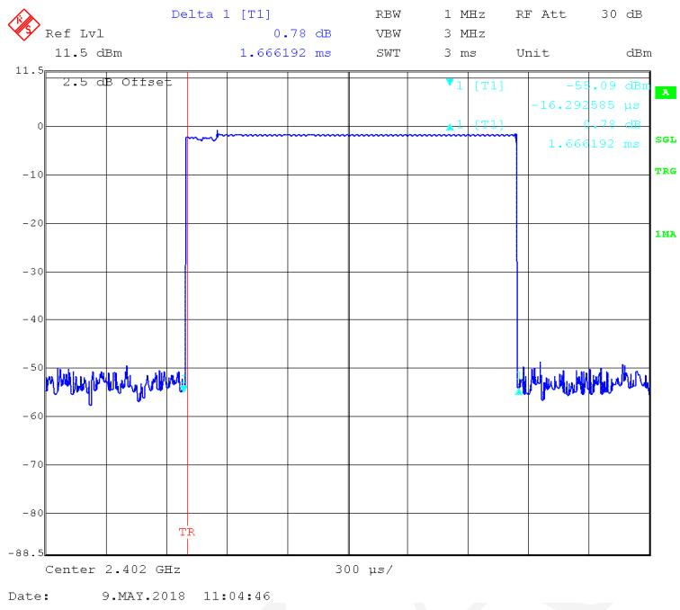
**EDR ( $\pi/4$ -DQPSK):Pulse time, Middle Channel, 2DH3**
