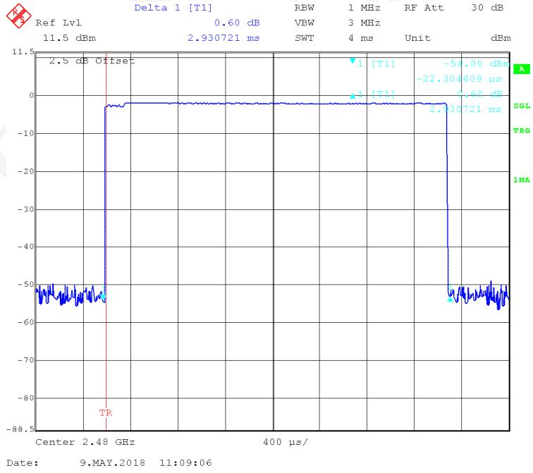
**EDR (8DPSK): Pulse time, Low Channel, 3DH1**
