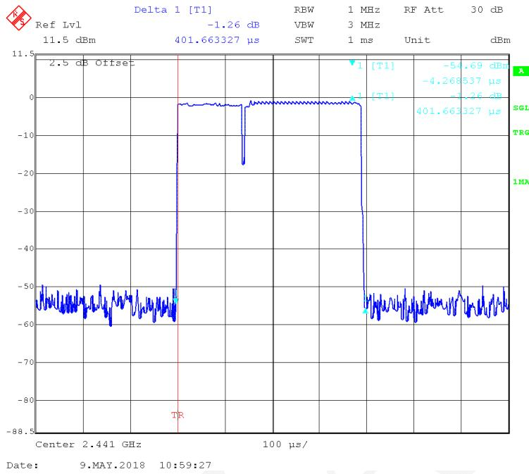
**EDR ( $\pi/4$ -DQPSK):Pulse time, High Channel, 2DH1**
