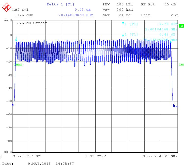
**EDR ( $\pi/4$ -DQPSK): Number of Hopping Channels**
