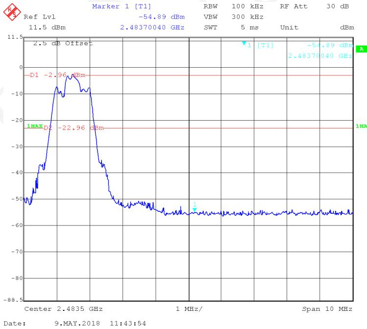
**EDR (8DPSK): Left Side**
