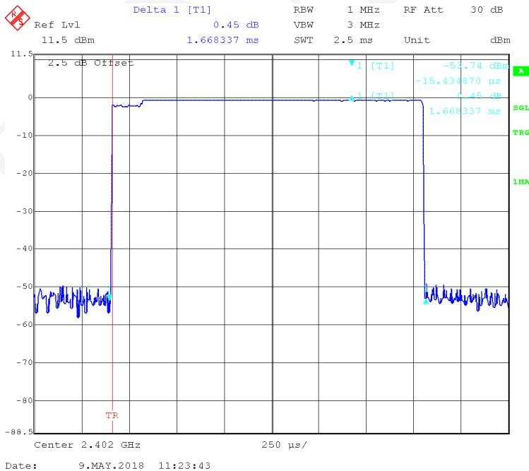
**EDR (8DPSK): Pulse time, Middle Channel, 3DH3**
