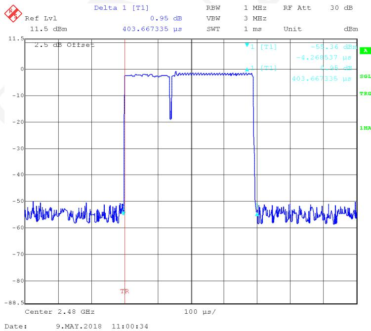
**EDR ( $\pi/4$ -DQPSK):Pulse time, Low Channel, 2DH3**
