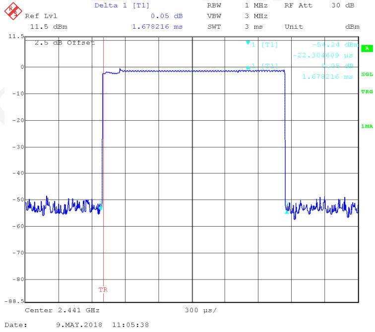
**EDR ( $\pi/4$ -DQPSK):Pulse time, High Channel, 2DH3**
