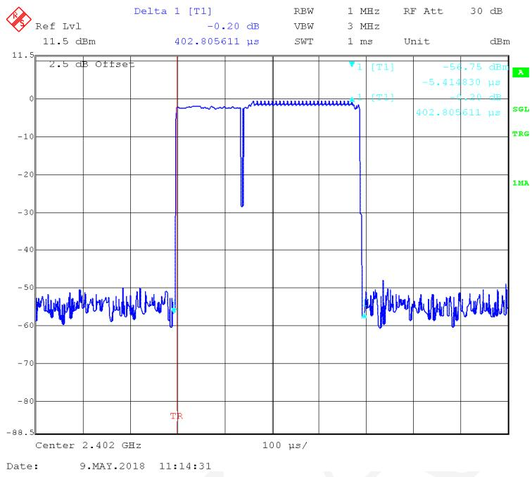
**EDR (8DPSK): Pulse time, Middle Channel, 3DH1**
