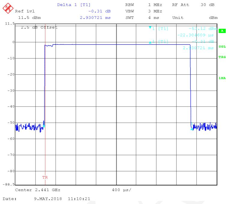
**EDR ( $\pi/4$ -DQPSK):Pulse time, High Channel, 2DH5**
