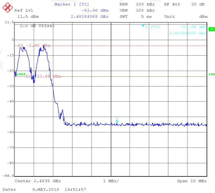
**EDR ( $\pi/4$ -DQPSK): Left Side - Hopping**
