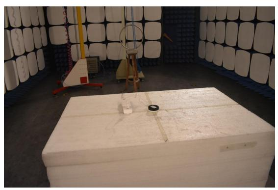
3. Radiated emission (9KHz-30MHz)
