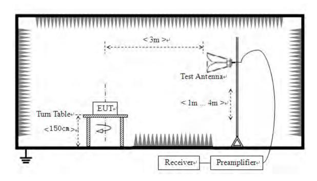
The RF absorbing material used on the reference ground plane and on the turntable have a maximum height (thickness) of 30 cm (12 in) and have a minimum-rated attenuation of 20 dB at all frequencies from 1 GHz to 18 GHz. Test site have a minimum area of the ground plane covered with RF absorbing material as specified in Figure 6 of ANSI C63.4: 2014.
