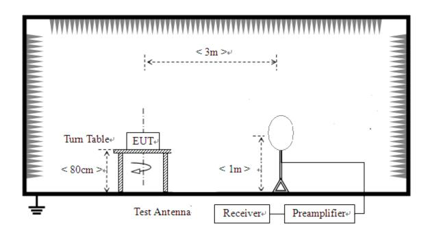
2) For radiated emissions from 30MHz to1GHz
