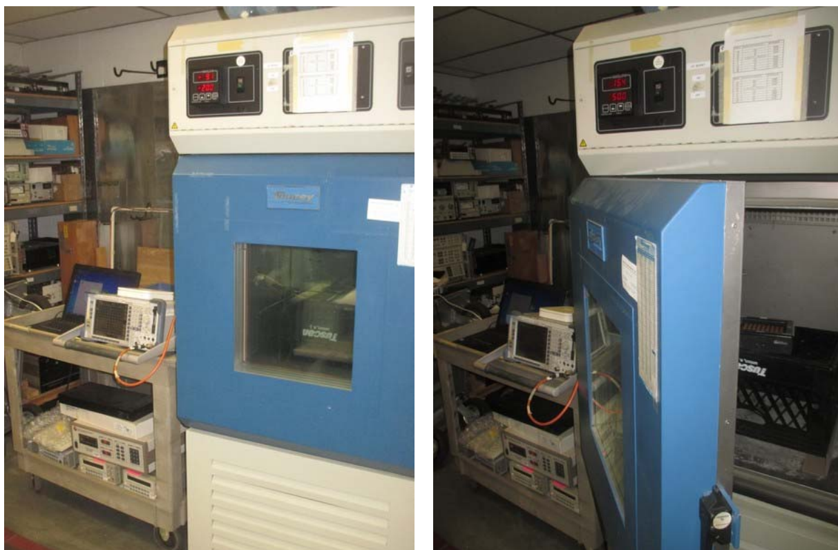
Figure 3.4 Frequency Tolerance Test Setup
