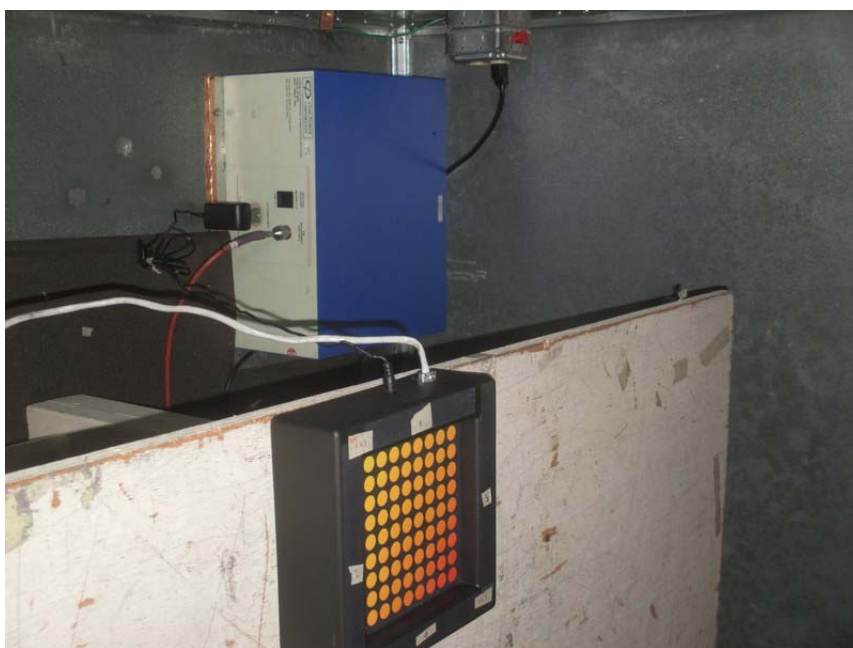
Figure 3.3 Conducted Emission Test Setup
