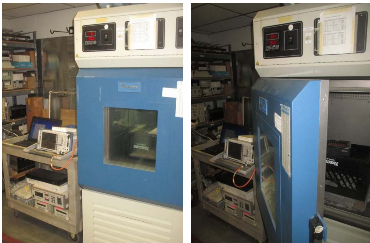
Figure 3.4 Frequency Tolerance Test Setup
