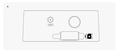
Gently pull the flap on its right side to reveal the Micro SIM card slot
