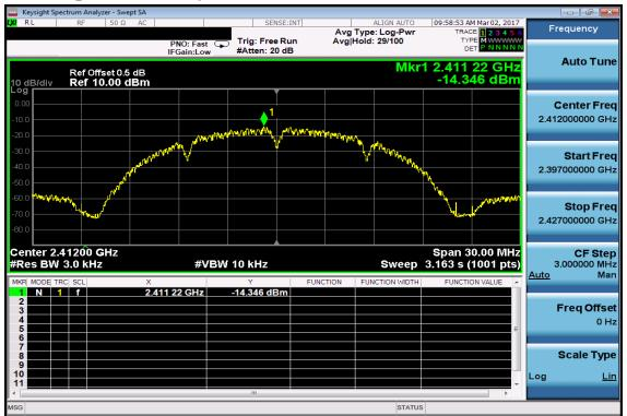
**Power Spectral Density Test Plot (CH-Mid)**
