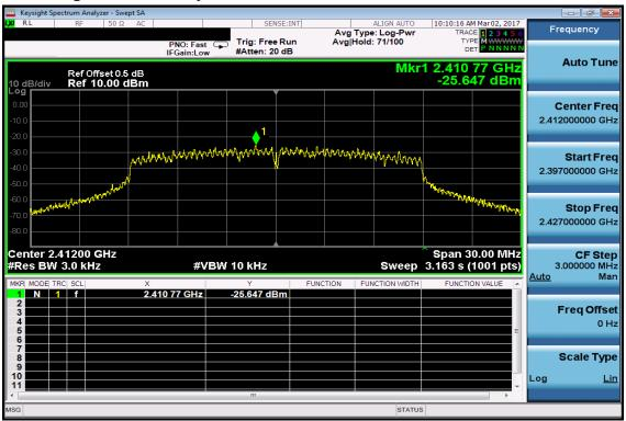
**Power Spectral Density Test Plot (CH-Mid)**
