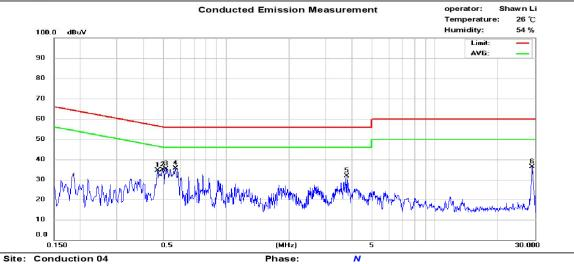
Limit: CISPR22 Class B Conduction(QP)
