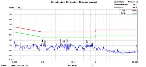
Limit: CISPR22 Class B Conduction(QP)
