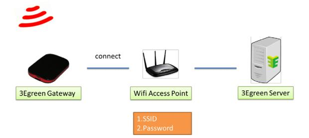
Gateway need connect with Wifi AP,then data can pass on sent to cloud servor. Gateway need know Wifi APSSID and Password, the Gateway APP function is to set the parameter into Gateway  $\circ$
